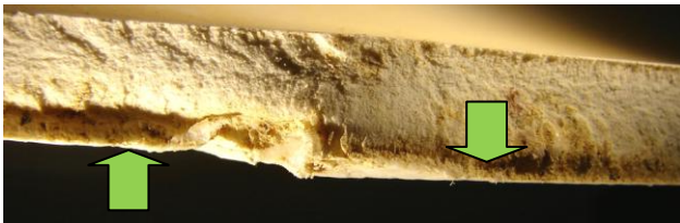
Figure 4: Digital image displaying the exterior rock impingement and fracture initiation area sectioned for SEM inspection. The rock-impingement location is generally bounded by the green arrows along the outside edge of the pipe which is down as shown in this photo. Note approximately 10-25% (thickness) penetration of the rock into the PVC pipe wall in wedge-like fashion.
