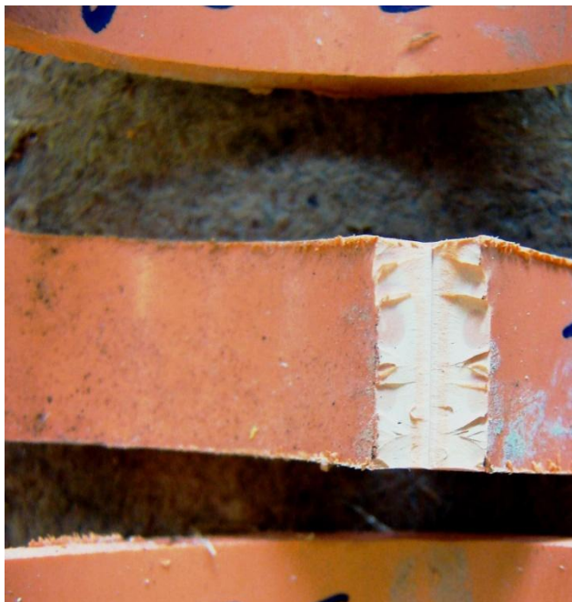
Figure 1: Digital image displaying a section cut from CPVC pipe with obvious brittle fracture zone. For scale, the pipe wall thickness is approximately 0.075 inches.
